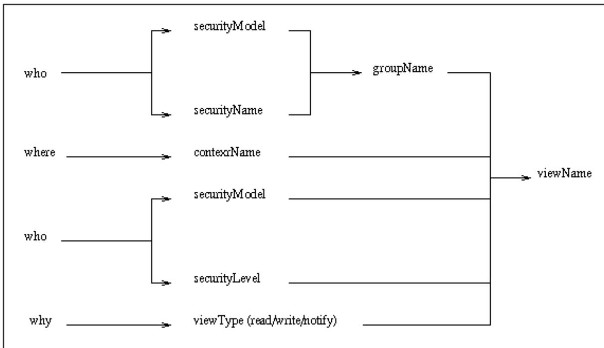
Figure 2.4: Overview of the mechanism of MIB selection
