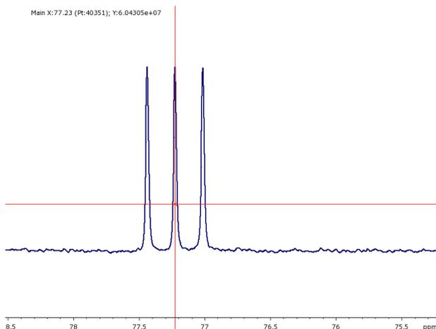
Using mouse again, shrink a spectrum a bit to see all peaks and use 'First order' phase correction sliced till all peaks have a pure absorption (positive) lineshapes.
