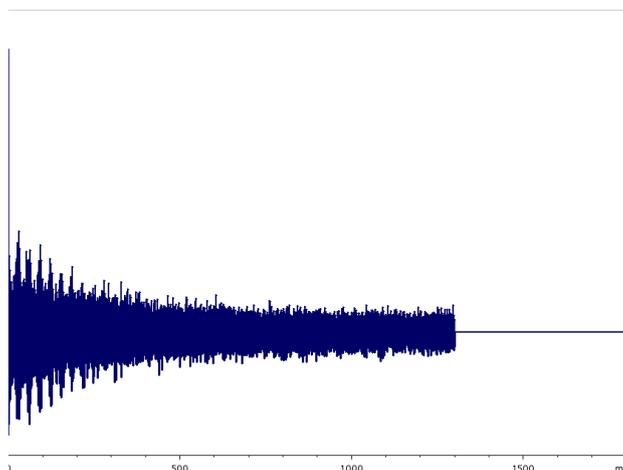
Pressing button with 'LB' label you will apply line-broadening (apodization) for the current FID. See specialised literature for details. Choose 'gaussian' type of broadening of 3 Hz linewidth in the prompt dialog:
